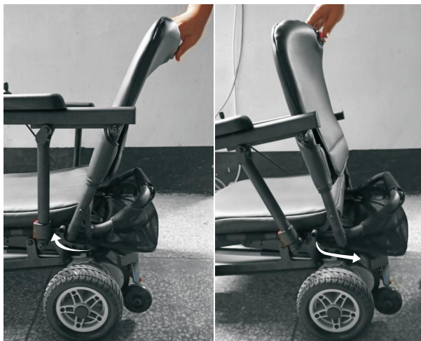
↑ Press the release button to adjust the seat back.
